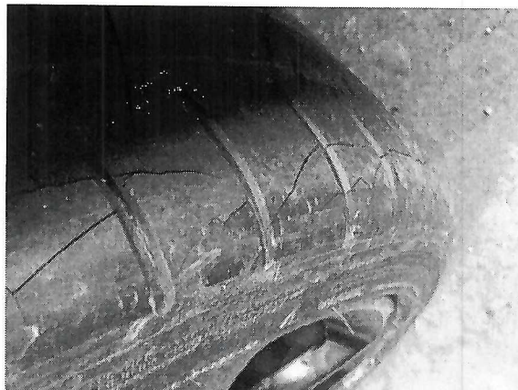
Photo 1: Cold Temperature Tire Damage (photo courtesy of Michelin Tires)
