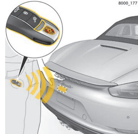
Fig. 124: Opening rear luggage compartment lid with Porsche Entry & Drive
