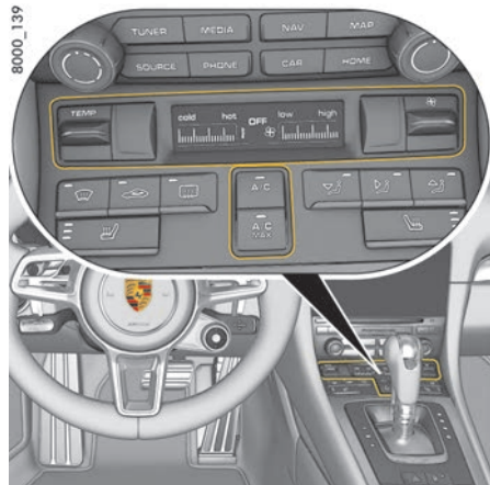
Fig. 12: Air-conditioning control panel
