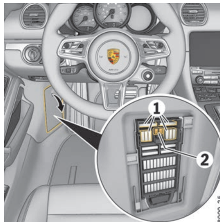
Fig. 87: Elements in the fuse box in the left footwell
