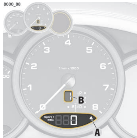
Fig. 225: Upshift indicator A and gear indicator B The consumption-orientated upshift indicator A helps the driver develop a fuel-saving driving style.
