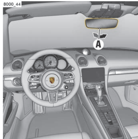
Fig. 134: Dimming interior mirrors manually
