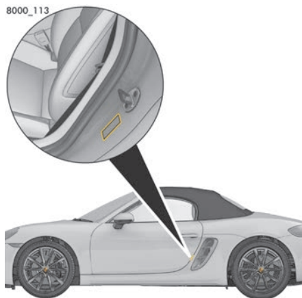
Fig. 231: Tyre pressure plate at the door sill area
