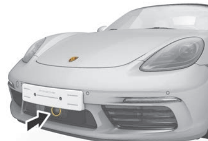
Fig. 1: Location of radar sensor
