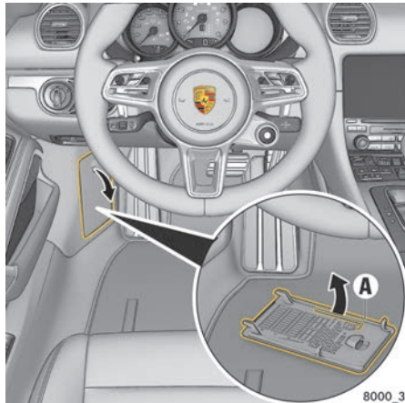
Fig. 79: Removing the metal hook
