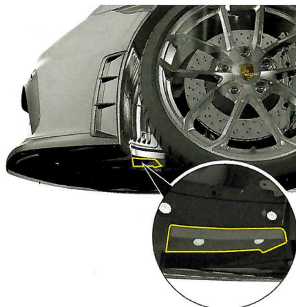
Fig. 6: Removing the insert from the diffuser duct
