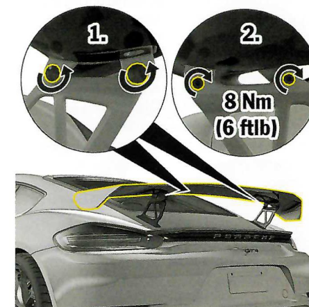
Fig. 5: Rear wing adjustment
