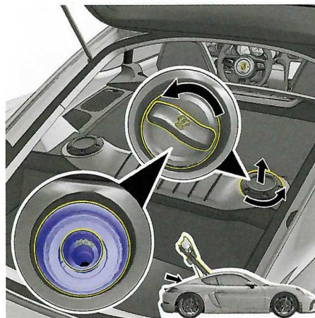
Fig. 8: Measuring the engine coolant level
